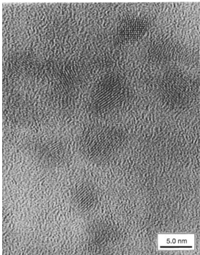
Figure 2. HRTEM images of CdSe nanocrystals overcoated with ZnSe. The [ZnSe/CdSe] ratio is \sim 2.5 .
